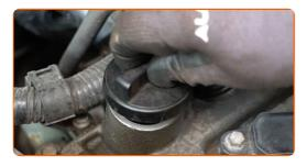
Tighten the oil filler cap.
