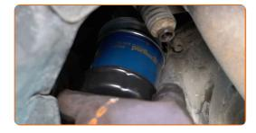
Tighten the oil filter. Remember to observe the recommended tightening torque. Use the 65-14F socket. Use a torque wrench. Tighten it to 24 Nm torque.
