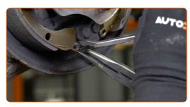
Remove the hold-down spring. Use a flat screwdriver.
