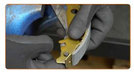
Reinstall the brake shoe hold-down cup. Use water pump pliers.
