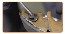
Remove the brake shoe adjuster lever. Use a flat screwdriver.
