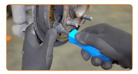
Remove the upper return spring of the brake shoes. Use round-nose pliers.
