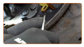
Install the hold-down spring. Use round-nose pliers.
