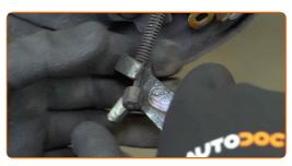
Perform further demounting of the upper retaining spring and the adjuster mechanism.
