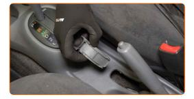
Loosen the parking brake cable. Use a drive socket #10. Use a ratchet wrench.
