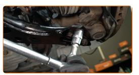
Tighten the brake caliper bracket fasteners. Use a drive socket #17. Use a torque wrench. Tighten it to 106 Nm torque.
