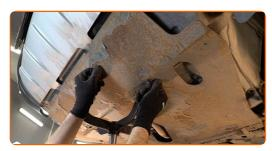
Tighten the fasteners of the oil pan lower cover. Use a drive socket #12.
