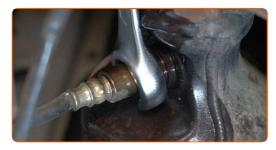
Remove the oxygen sensor.
