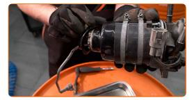
Screw in the bracket of the water-in-fuel sensor. Use a drive socket #8. Use a ratchet wrench.
