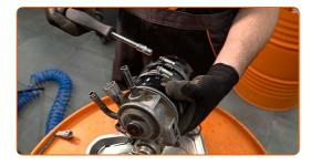
Remove the O-ring of the water-in-fuel sensor. Use a flat screwdriver.
