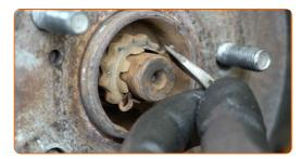
Remove the wheel hub bearing retaining ring. Use a crowbar.
