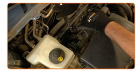
23 Install the panel assembled with the windscreen wiper linkage.
