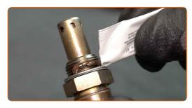
Install the new oxygen sensor.
