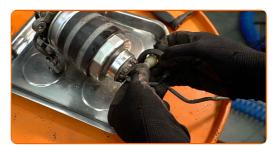
10 Unscrew the water-in-fuel sensor.
