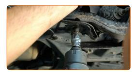
Remove the rear fastener of the control arm.
