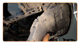
Tighten the fasteners of the oil pan lower cover. Use a drive socket #10. Use a ratchet wrench. Use a clip removal tool.
