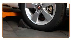
Loosen the wheel mounting bolts. Use wheel impact socket #21.
