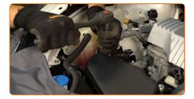
Screw in the coolant reservoir fasteners. Use a drive socket #14. Use a ratchet wrench.
