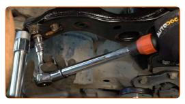
Remove the support from under the arm.
