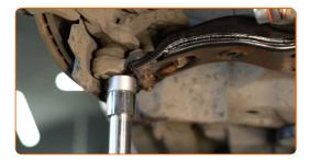
Tighten the front fastener connecting the control arm to the subframe. Use a drive socket #22. Use a torque wrench. Tighten it to 233 Nm torque.
