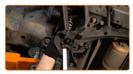
Tighten the ball joint fastener. Use a drive socket #17. Use a torque wrench. Tighten it to 89 nm torque.
