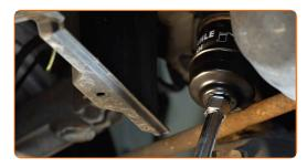
Prepare a container for the old oil filter. Put the old oil filter in the container. 10
