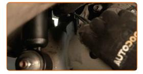
Unscrew the hub bearing mounting. Use a drive socket #10. Use a ratchet wrench. Use a tap wrench.
