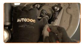
Disconnect the ABS sensor wiring.
