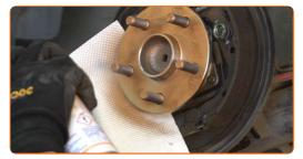
20 Install the brake drum and fasten it.
