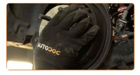
Tighten the fastener of the wheel hub bearing. Use a drive socket #10. Use a torque wrench. Tighten it to 61 nm torque.
