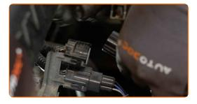
Unfasten the clamp to release the oxygen sensor wiring harness. Use a flat screwdriver.
