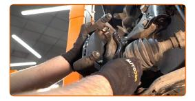
Tighten the brake caliper bracket. Use a drive socket #17. Use a torque wrench. Tighten it to 98 Nm torque.
