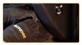
A Remove the cabin filter housing cover.
