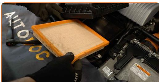
**7** Cover the air intake hose with a microfibre towel to prevent dust and dirt from getting into the system.
