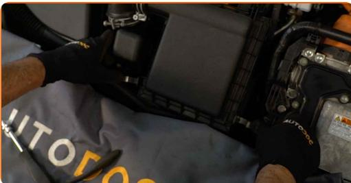
**5** Slightly raise the cover of the air filter housing.
