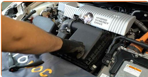
**12** Press the air filter cover clips into place.
