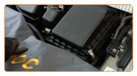
Fasten the clamp on the air intake hose. Use a drive socket #10. Use a ratchet wrench.
