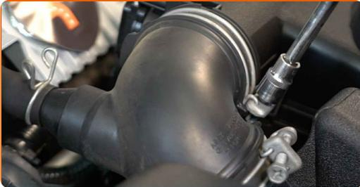
**4** Release the air filter cover clips.
