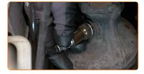
Tighten the oxygen sensor fastener. Use a 22-mm oxygen sensor socket. Use a torque wrench. Tighten it to 40 Nm torque.
