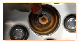
Tighten the wheel bolts using a criss-cross pattern. Use a torque wrench. Tighten it to 103 Nm torque.
