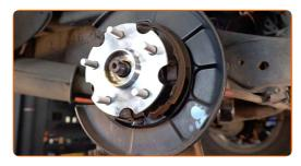
Tighten the wheel hub bearing fasteners. Use a drive socket #17. Use a ratchet wrench.
