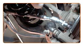
Remove the caliper bracket.
