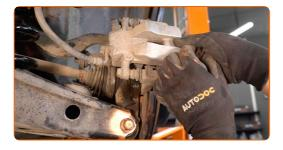
Tighten the brake caliper bracket. Use a drive socket #18. Use a torque wrench. Tighten it to 88 nm torque.
