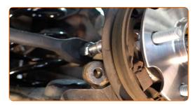
Tighten the fastener of the wheel hub bearing. Use a drive socket #17. Use a torque wrench. Tighten it to 90 nm torque.
