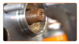
Screw the nut of the drive shaft. Use a drive socket #30. Use a tap wrench.
