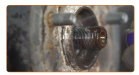
Remove the drive shaft. Use a pin punch. Use a hammer.
