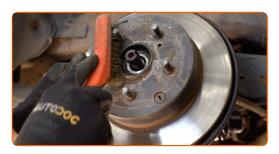
17 Remove the brake disc.
