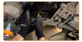
Screw the rear fastener connecting the control arm to the subframe. Use a combination spanner #22. Use a drive socket #22. Use a ratchet wrench.
