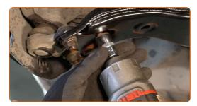
Install the rear fastener of the arm.
