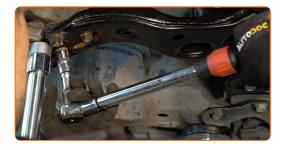
Remove the support from under the arm.
