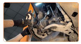
15 Remove the brake disc.
