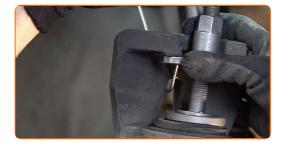
Install the brake caliper and fix it. Use a drive socket #14. Use a torque wrench. Tighten it to 35 Nm torque.
