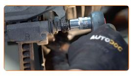
10 Remove the brake caliper.
