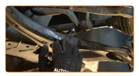
Unscrew the fastener connecting the stabilizer link to the shock strut. Use a combination spanner #17. Use a drive socket #17. Use a ratchet wrench.
