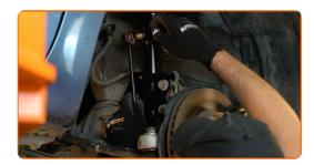
Tighten the fastener connecting the stabilizer link to the shock strut. Use a drive socket #19. Use a torque wrench. Tighten it to 74 Nm torque.
