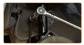
Tighten the fastener connecting the stabilizer link to the stabilizer bar. Use a drive socket #19. Use a torque wrench. Tighten it to 74 Nm torque.
