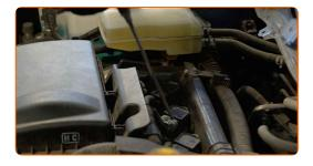
Unscrew the fasteners of the ignition coils. Use a drive socket #10. Use a ratchet wrench.
