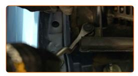
Treat the fasteners of the windscreen wiper linkage. Use WD-40 spray.
