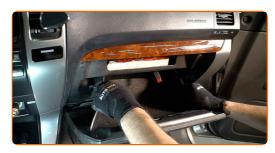
Remove the cabin air filter housing.
