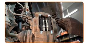
Install the retaining spring of the brake pads.
