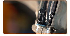
Install the brake pads retaining clips.
