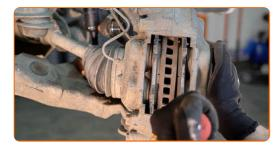
12 Remove the brake pads.
