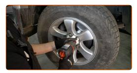
Lower the car and working in a cross order, tighten the wheel bolts. Use a torque wrench. Tighten it to 112 Nm torque.
