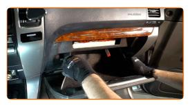
Remove the cabin air filter housing.
