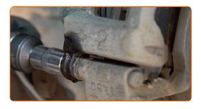
10 Remove the brake caliper.
