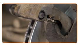
Treat the brake caliper piston. Use a wire brush. Use a brake cleaner.
