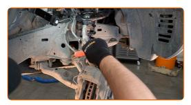
Disconnect the brake hose mounting bracket. Use a drive socket #12. Use a ratchet wrench.
