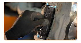
Install the retainer of the brake pads. Use a crowbar. Use a rubber mallet.
