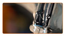
Install the brake pads retaining clips.
