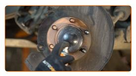
21 Install the brake disc.
