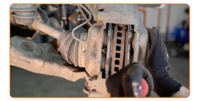
12 Remove the brake pads.
