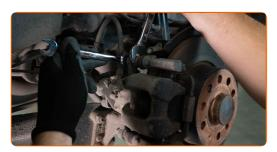
10 Remove the brake caliper.
