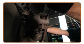
Clean the brake caliper bracket fasteners. Use a wire brush. Treat the brake caliper bracket fasteners. Use WD-40 spray.
