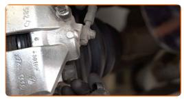
20 Install the brake caliper retaining spring.
