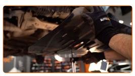
Tighten the fasteners of the oil pan lower cover. Use a drive socket #12.
