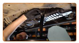
Replacement: engine oil and filter – VW Transporter T4. Tip from AUTODOC experts:
