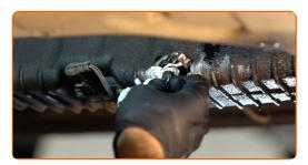
Screw in the new drainage plug and tighten it. Use a drive socket #17. Use a torque wrench. Tighten it to 30 nm torque.
