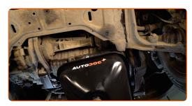
Unscrew the drain plug. Use a drive socket #17. Use a ratchet wrench.
