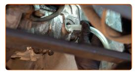
Pour the oil into the gearbox through the filler hole. Required amount of oil: 2.5 L.
