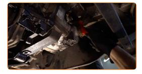
6.2 Clean the area of the oil pan drainage hole. Use a wire brush. Use WD-40 spray.
