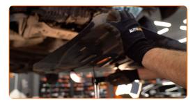
Tighten the fasteners of the oil pan lower cover. Use a drive socket #12. Use a Phillips screwdriver. Lower the car.
