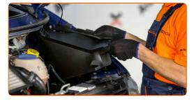
Remove the fender protection cover.
