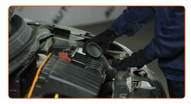
6 Remove the air filter housing.
