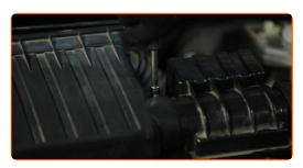
28 Press the air filter cover clips into place.
