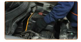
Unscrew the engine cover fastener. Use a drive socket #8. Use a ratchet wrench.
