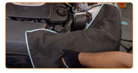
Release the air filter cover clips. Use a flat screwdriver.
