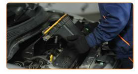
Connect the air intake pipe to the air filter housing.
