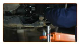
Tighten the lower fastener of the shock absorber. Use a drive socket #17. Use a torque wrench. Tighten it to 90 Nm torque.
