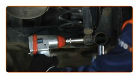
Detach the lower part of the shock absorber. Use a flat screwdriver.
