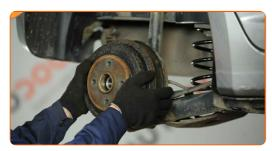
Tighten the hub. Use a drive socket #30. Use a torque wrench. Tighten it to 175 Nm torque.
