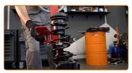
Tighten the shock strut piston rod nut. Use a combination spanner #19. Use HEX No.H6. Use a torque wrench. Tighten it to 50 Nm torque.
