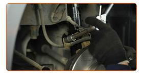
Connect the ABS sensor wiring.
