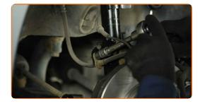
Remove the bracket from the shock absorber strut.
