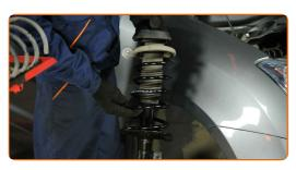
Screw the top fastening of the shock strut mount.
