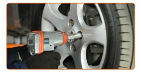
Lower the car and working in a cross order, tighten the wheel bolts. Use wheel impact socket #21. Use a torque wrench. Tighten it to 85 nm torque.
