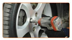
Lower the car and working in a cross order, tighten the wheel bolts. Use wheel impact socket #21. Use a torque wrench. Tighten it to 85 nm torque.
