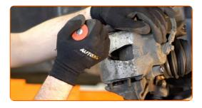
10 Remove the brake caliper.
