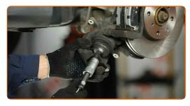
17.1 Install the brake caliper and fix it.
