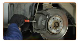
10 Remove the brake caliper.
