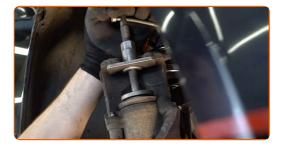
35.1 Install the brake caliper and fix it.
