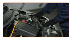
Remove the air filter housing.
