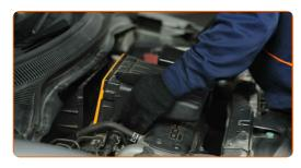
Unscrew the engine cover fastener. Use a drive socket #8. Use a ratchet wrench.
