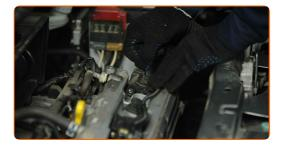
Install the spark plug wire connectors into the spark plug wells. Make sure you hear a click indicating that it is locked in place.
