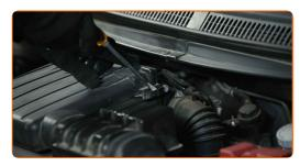
Unscrew the air filter housing fastener. Use a drive socket #10. Use a ratchet wrench.
