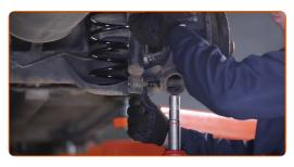
Remove the support from under the stub axle.
