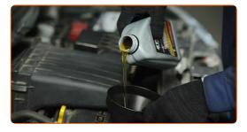
Replacement: engine oil and filter – SUZUKI SUPER CARRY Bus (ED). Tip from AUTODOC:
