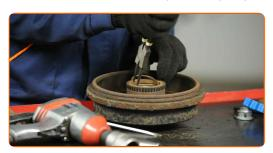
16 Install the brake drum assembled with the wheel hub bearing.
