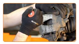
10 Remove the brake caliper.
