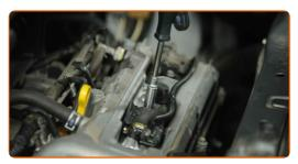
Unplug the connectors from the ignition coils. Use a flat screwdriver.
