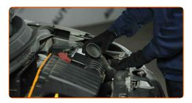
Remove the air filter housing.
