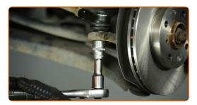
Tighten the tie rod end locknut. Use a combination spanner #19. Use a torque wrench. Tighten it to 65 nm torque.
