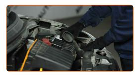
Remove the air filter housing.
