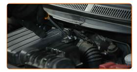
Unscrew the air filter housing fastener. Use a drive socket #10. Use a ratchet wrench.
