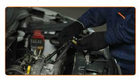
Replacement: spark plugs – SUZUKI Grand Vitara II Off-Road (JT, TE, TD). Tip from AUTODOC:
