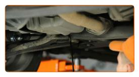
Replacement: engine oil and filter – SUZUKI Carry Platform / Chassis (FD, DA5\_T, DA6\_T). Tip:
