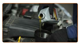
Replacement: engine oil and filter – SUZUKI Carry Platform / Chassis (FD, DA5\_T, DA6\_T). Tip from AUTODOC:
